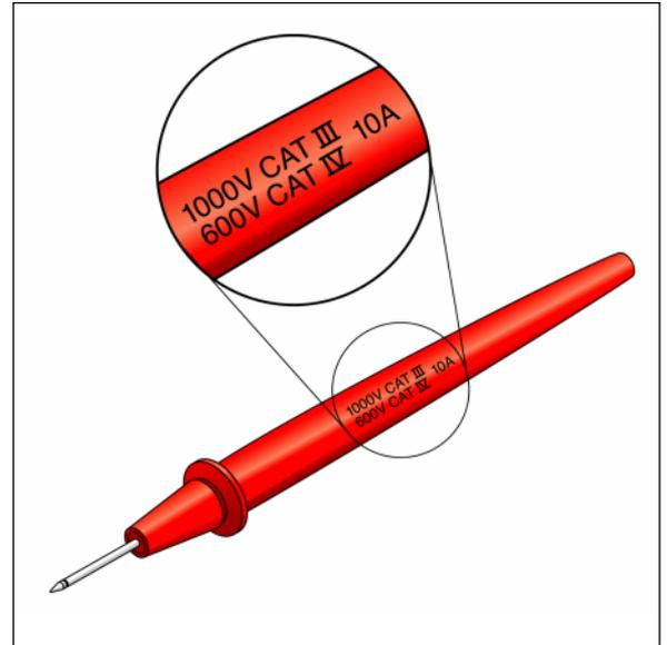
though the DMM is clearly marked with this safety rating, are the test leads equally rated? If the DMM's test leads do not equal or exceed the rating of the tester, then you are putting the tester, and more importantly, yourself at risk.
