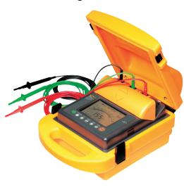
Digital insulation testing up to 5000 volts The Fluke 1550B is a digital insulation tester capable of testing switchgear, motors, generators and cables at up to 5000 V DC. It can be used for a wide range of tests: from simple spot checks to timed tests and breakdown tests. Measurement storage and PC interface software make it ideal for preventive maintenance. Heavy-duty leads, probes and alligator clips fit in the custom carrying case, for a rugged field testing kit.
