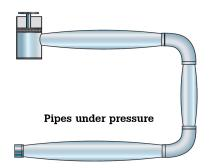
An electrical system is like a plumbing system, where voltage is like fluid pressure, current is like fluid flow rate, resistance is like a shut-off valve and electrical insulation is like the walls of the pipe. If there is corrosion in the wall of the pipe water will leak
