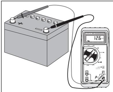
**Figure 1: Measuring System Voltage**
