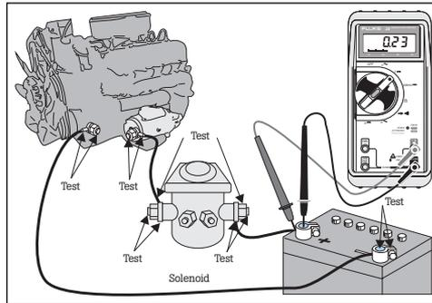
**Figure 8: Testing for excessive voltage drop**
