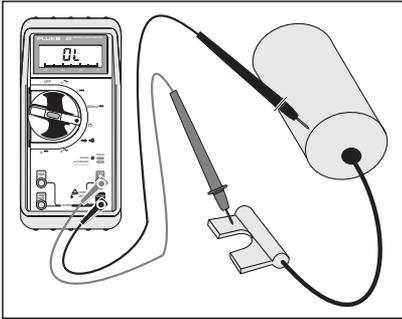
**Figure 10: Checking condenser leakage**
