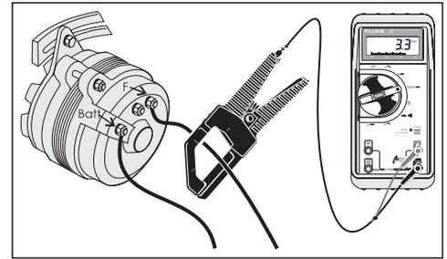
**Figure 4: Checking field current**
