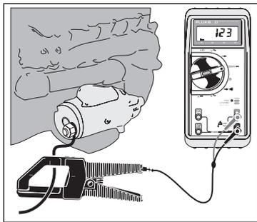
**Figure 7: Measuring starter current draw**
