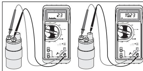
**Figure 9: Measuring internal coil resistance**
