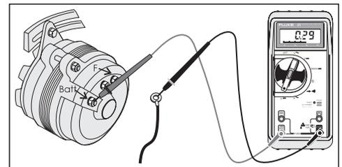
**Figure 6: Alternator leakage current**
