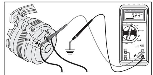
**Figure 5: Checking ripple voltage**
