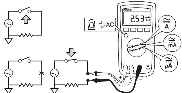
**Figure 2. Measuring AC and DC Current**
