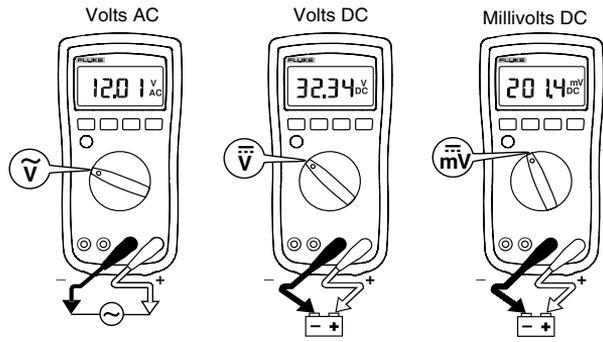
**Figure 1. Measuring AC and DC Voltage**
