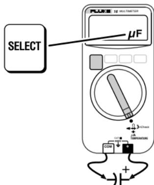
If the capacitor requires more discharging, **diSC** is displayed while the capacitor discharges.
