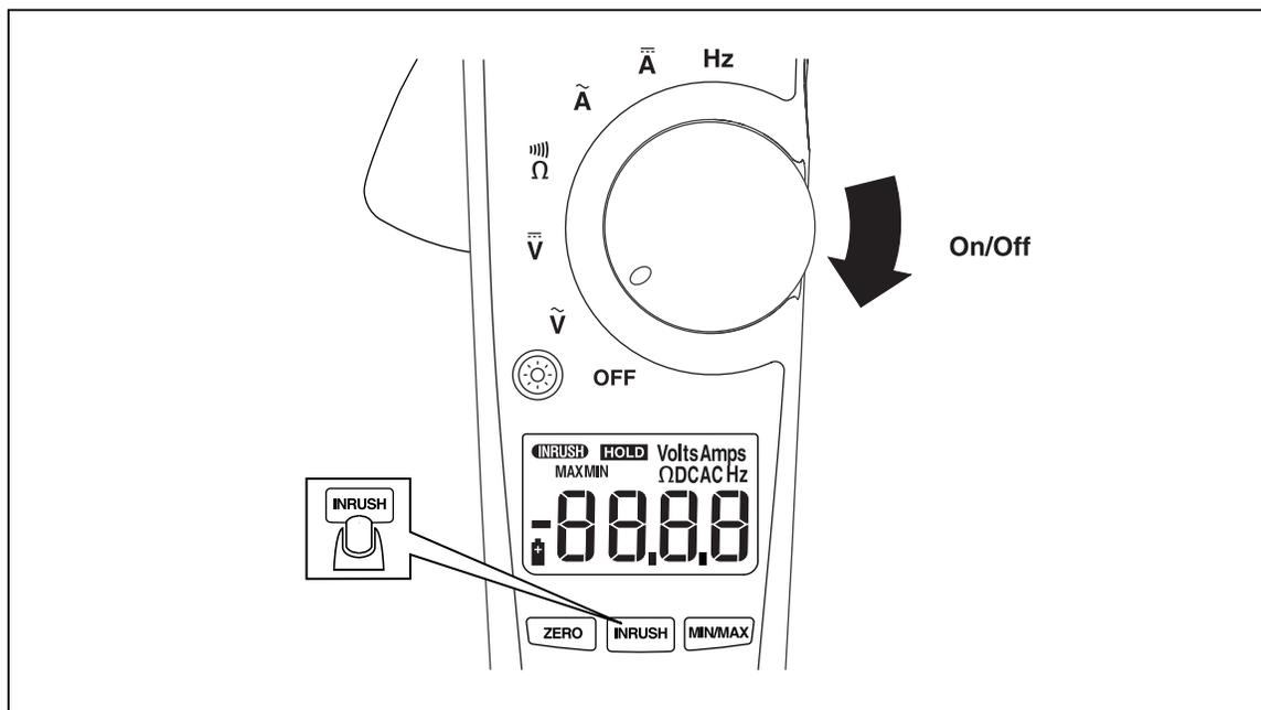
**Figure 2. Testing the Display (337 is shown)**
