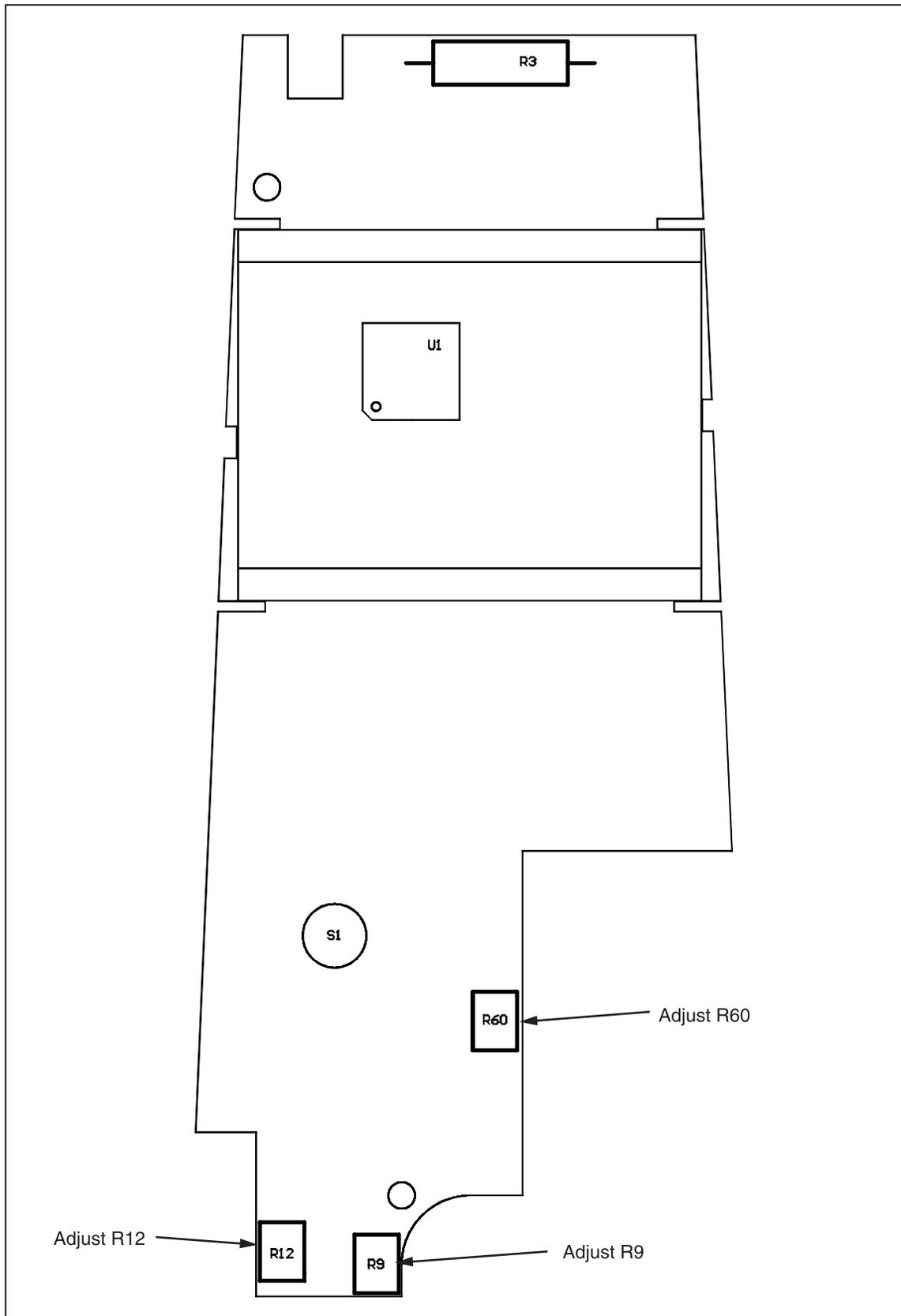
**Figure 6. Calibration Adjustment Points 336-337**
