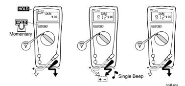
When the meter captures new input, it beeps and a new reading is displayed.
