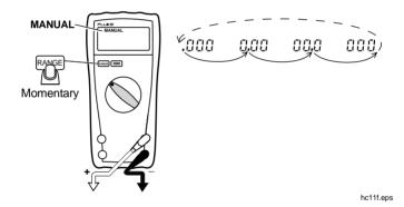
To return to autorange, press  $\boxed{\text{RANGE}}$  for 1 second or turn the rotary switch.
