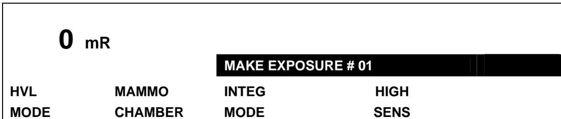
Make the first exposure with no filtration in the beam.
