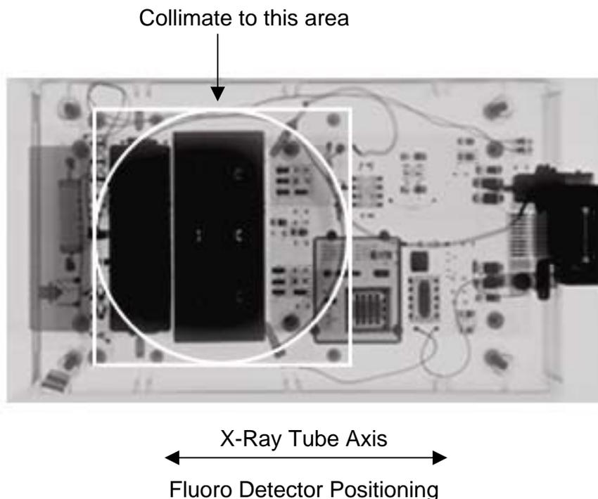
For automatic brightness control machines, place appropriate shielding over the detector to drive the output to its maximum. A folded lead apron, gloves or a lead sheet may be used. For manual systems, set the machine for its maximum output and use appropriate shielding to protect the image intensifier.
