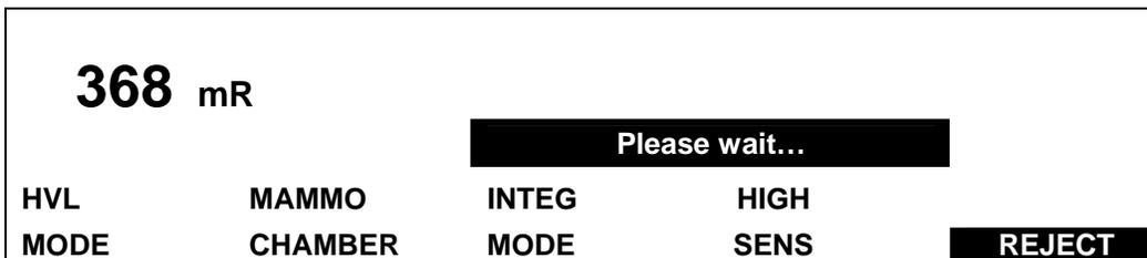
The exposure data from the first exposure is displayed and the NERO mAx prepares to take the second exposure. Please wait while the NERO mAx prepares to take the next exposure. If the NERO mAx detects a fault condition such as a high offset, an error message is displayed and the user must correct the error to continue (see Section 4.3--Error Messages--for more information).
