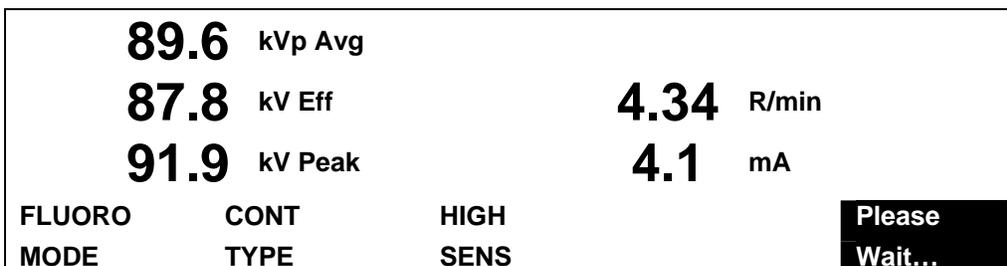
After data analysis is complete, kV, exposure rate and mA are displayed. If an overrange is detected an error message is displayed. If the calculated kV is above or below the selected filter kV range, "High" or
