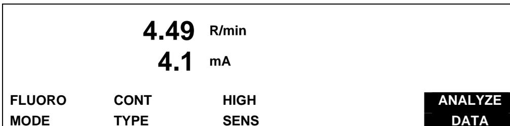
After the beam is turned off, the NERO mAx analyzes the fluoro exposure kV data.
