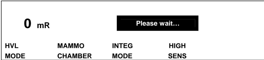
Please wait while the NERO mAx prepares to take an exposure. If the NERO mAx detects a fault condition such as a high offset, an error message is displayed and the user must correct the error to continue (see Section 4.3--Error Messages--for more information). When the NERO mAx is ready to take an exposure it will beep and prompt for an exposure.
