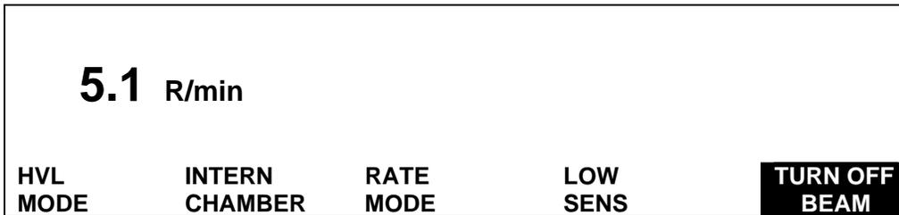
Turn off the x-ray beam. The NERO mAx has stored the measured exposure rate and will set up for the next exposure as soon as the beam turns off.
