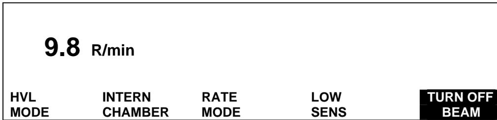
Turn off the x-ray beam. The NERO mAx has stored the measured exposure rate and will set up for the next exposure as soon as the beam turns off.
