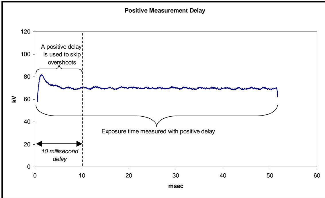
An example showing this use of a measurement delay can be found in troubleshooting Section 4.5-- Waveforms - Overshoot.
