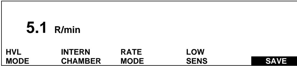
After the second exposure has started, the NERO mAx displays the exposure rate. When the rate has stabilized or the desired rate has been achieved, press the SAVE softkey (softkey 4) to save the rate measurement.
