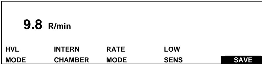
After the exposure has started, the NERO mAx displays the exposure rate. When the rate has stabilized or the desired rate has been achieved, press the **SAVE** softkey (softkey 4) to save the rate measurement.
