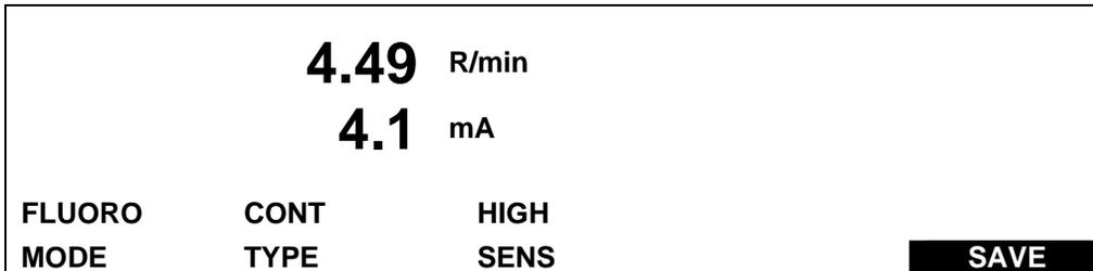
After the exposure starts, the NERO mAx displays exposure rate and mA. When the desired exposure rate and/or mA are displayed, press the SAVE key to acquire kV data.
