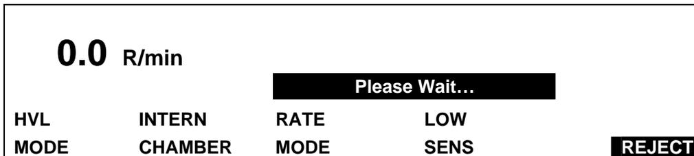
While the exposure rate from the first exposure is displayed, the NERO mAx prepares to take the second exposure. Please wait while the NERO mAx prepares to take the next exposure. If the NERO mAx detects a fault condition such as a high offset, an error message is displayed and the user must correct the error to continue (see Section 4.3--Error Messages--for more information).
