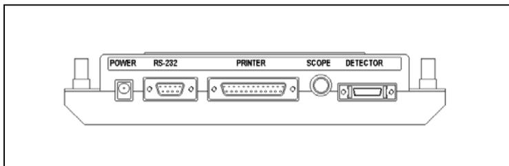
Figure 1-2. Control Console Rear Panel
