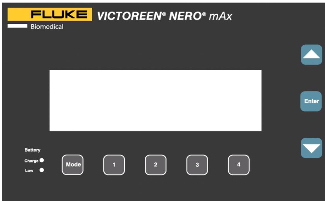
The NERO mAx display is divided into 5 columns, each column corresponds to the push button (softkey) directly beneath it. The left most column is the "MODE" column that is used to select the NERO mAx's operating mode. The remaining four columns (1 through 4) display various options for each mode.
