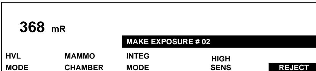
The NERO mAx is now ready to take the next exposure. Position an aluminum absorber in the beam and make the exposure. If the previously measured exposure is not acceptable, press the reject softkey to retake the exposure. If an overrange occurs, an error message is displayed and the exposure must be taken over.
