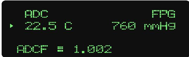
Figure 2-12. The Air Density Screen With Air Density Corrections Enabled
