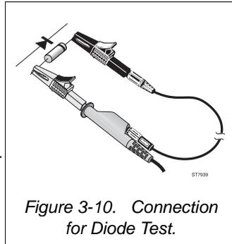
Figure 3-10. Connection for Diode Test.
