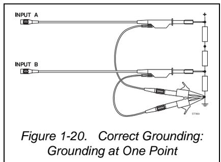
*Figure 1-20. Correct Grounding: Grounding at One Point*
