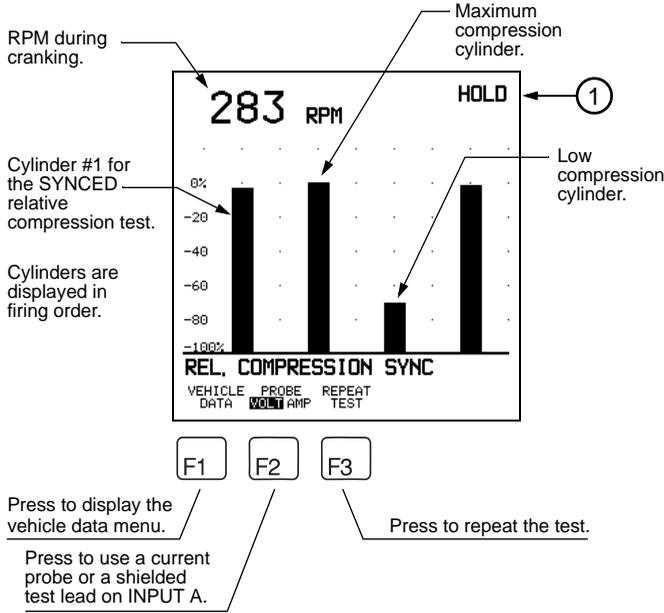
Figure 3-8. Relative Compression Test on a 4-Cylinder Engine.
