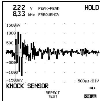
Figure 5-36. Result Display from a Knock Sensor Test
