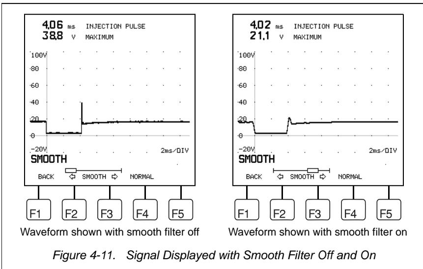
Figure 4-11. Signal Displayed with Smooth Filter Off and On
