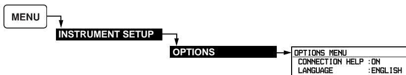
**CONNECTION HELP:** Can be set On (default) or Off. This setting is used to enable or disable display of connection help information during selection of a test.
