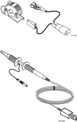
Used for RPM, injection pattern analysis, and advance tests on diesel engines with 6 mm fuel pipes. This set consists of a Piezo Pickup, which is clamped on the fuel pipe, a Probe-to-Piezo Pickup Adapter, a Low Pass Filter Probe to be connected to the test tool, and some additional accessories (not shown). Also see Appendix 7B under 'Optional Accessories'.
