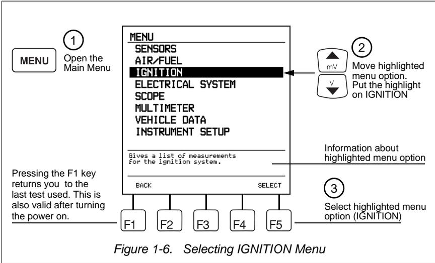
Subsequently follow steps ① and ② in Figure 1-7 to select SECONDARY IGNITION test.
