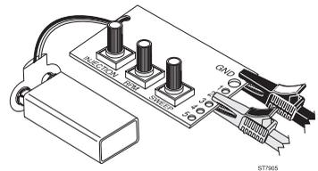
For this measurement we use the red test lead, since the Demo Board is not able to generate a high voltage secondary signal. Connect the red test lead to INPUT A, the red alligator clip to TP 2 (SEC. IGN.), and the black alligator clip to the GND connection of the Demo board.
