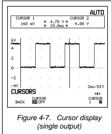
Figure 4-7. Cursor display (single output)
