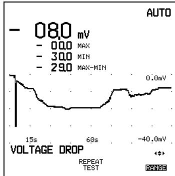
Figure 5-57. Result Display from a Voltage Drop Test
