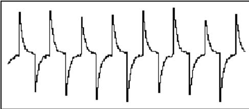
Idle Air Bypass waveforms may have unique shapes such as these and have a saw-curved appearance due to inductance reactance.
