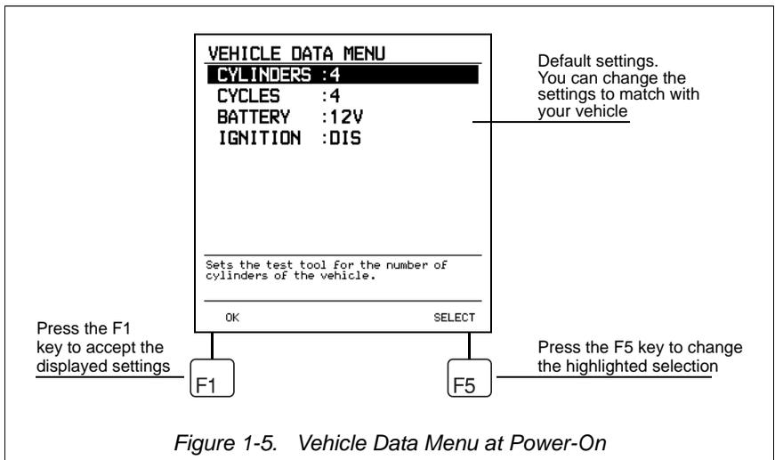
Figure 1-5. Vehicle Data Menu at Power-On
