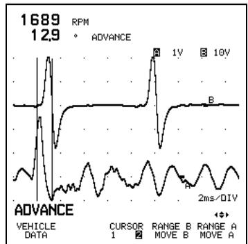
Figure 5-64. Advance at 1700 RPM.
