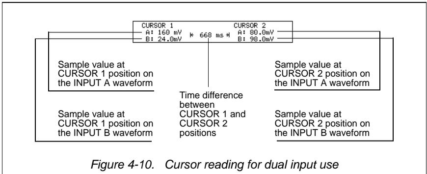
Figure 4-10. Cursor reading for dual input use
