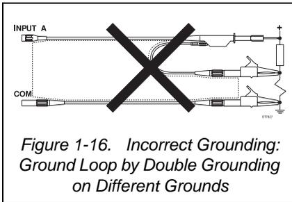
*Figure 1-16. Incorrect Grounding: Ground Loop by Double Grounding on Different Grounds*
