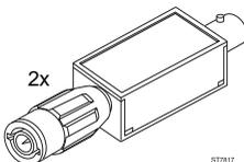
Used for oxygen sensor tests to provide 10 MΩ/3.5pF input impedance. This low-pass Filter Adapter eliminates noise over 4 kHz. One side of the adapter is connected to INPUT A or B, the other side is used to connect the shielded test lead.
