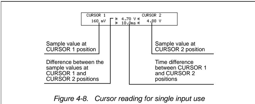
Figure 4-8. Cursor reading for single input use
