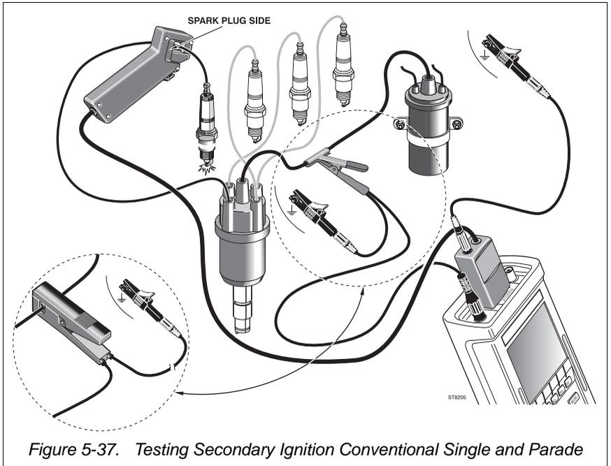
Figure 5-37. Testing Secondary Ignition Conventional Single and Parade
