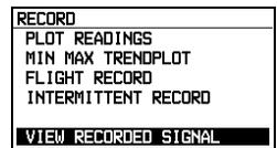
When you enter VIEW RECORDED SIGNAL, the display shows the readings that were on the display at the time you stopped recording. A vertical cursor appears at the location where these readings are valid, that is, at the end of the record. (See Figure 4-2)
