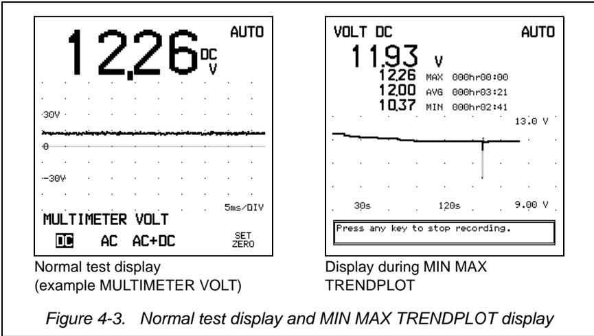
The graphical plot is displayed in the same way as PLOT READINGS, except in this function, time base rescaling does not stop after 16 minutes. Recording stops when you press any key on the Automotive ScopeMeter test tool.
