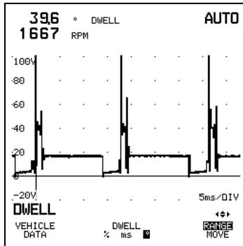
Figure 5-43. Result Display from a Dwell Test
