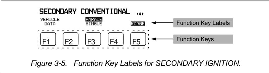
Figure 3-5. Function Key Labels for SECONDARY IGNITION.
