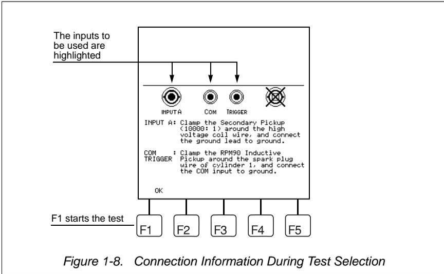
Press **F1** to start the test. For this example, it is not necessary to make the actual connections.
