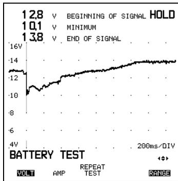
Figure 5-51. Result Display from a Battery Condition Test
