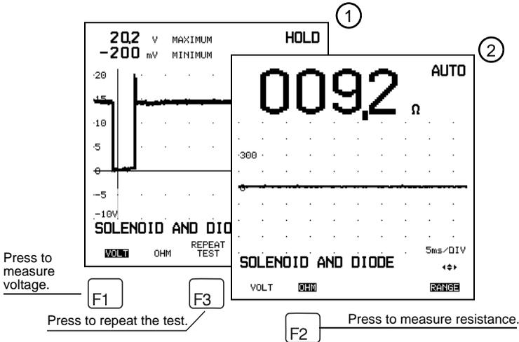
For the voltage test (F1 key), this is a single shot measurement, which means that the signal is displayed only once. To get a new test result, press the F3-key and reapply the signal from the solenoid.
