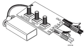
For this measurement, the battery is connected to the Demo Board. Connect the red test lead to INPUT A, the red alligator clip to TP 3 (potentiometer slider), and the black alligator clip to the GND of the Demo Board.
