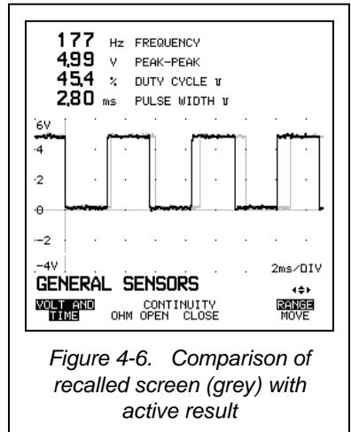
Figure 4-6. Comparison of recalled screen (grey) with active result
