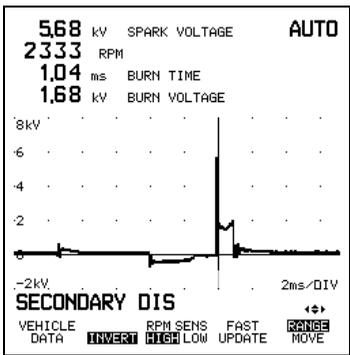
Use the F3 key to set the optimal RPM SENSitivity level:
