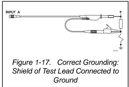
*Figure 1-17. Correct Grounding: Shield of Test Lead Connected to Ground*
