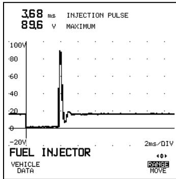
Figure 5-29. Result Display from a Fuel Injector Test
