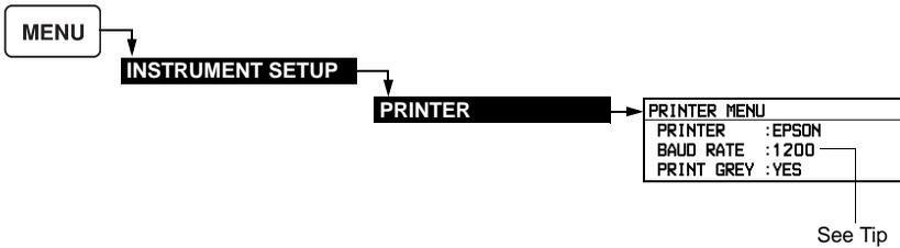
**PRINTER:** Defines the type of printer connected to the test tool.
