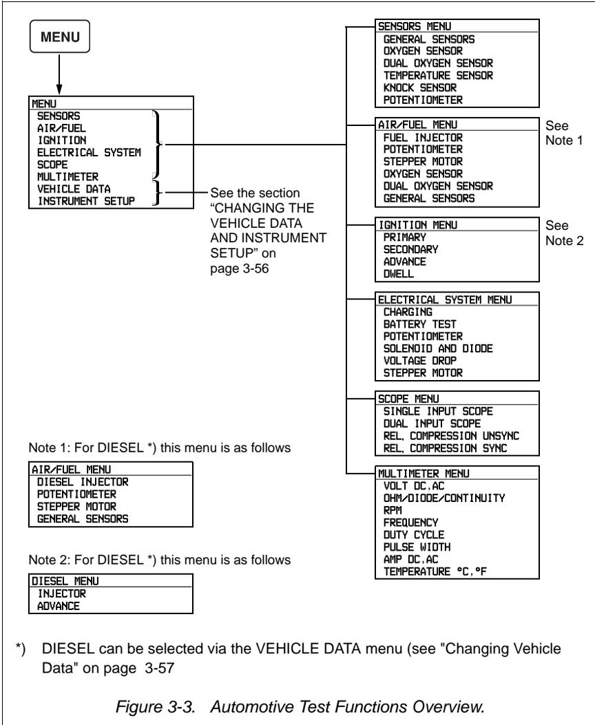
Figure 3-3. Automotive Test Functions Overview.
