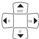
When you press one of the arrow keys, the test tool switches to manual control of range (timebase and vertical range) and trigger settings.
