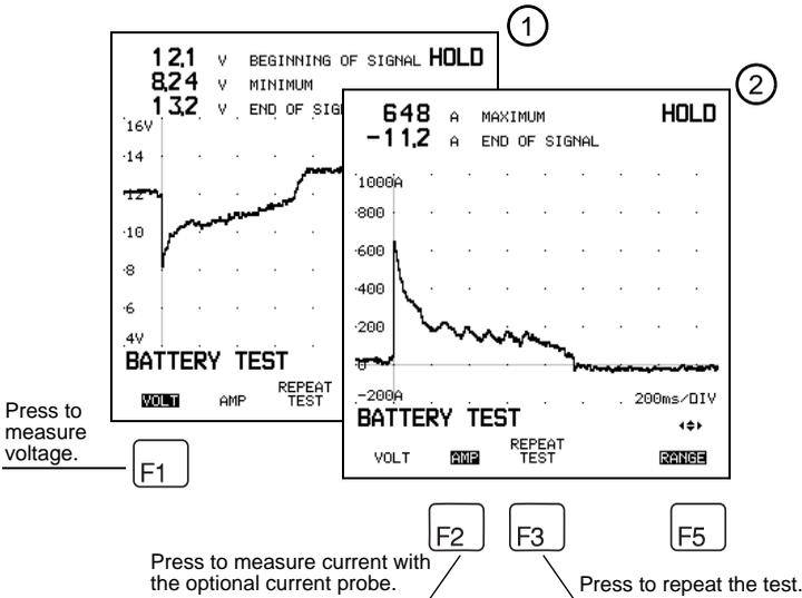
This test is a single shot measurement, which means that the signal is displayed only once. To get a new test result, stop the engine, press the F3-key and crank the engine again.
