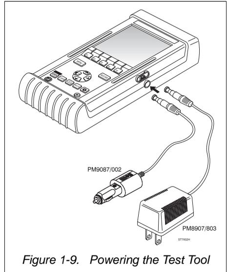
Figure 1-9. Powering the Test Tool
