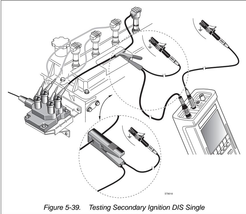
Figure 5-39. Testing Secondary Ignition DIS Single
