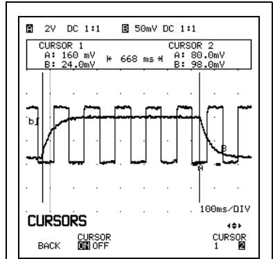
Figure 4-9. Cursor display (dual output)
