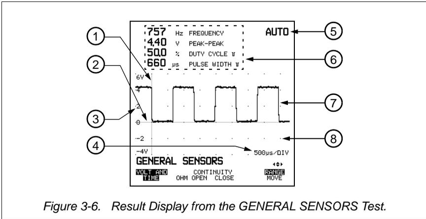
Figure 3-6. Result Display from the GENERAL SENSORS Test.
