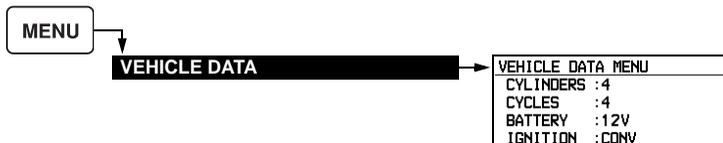
**CYLINDERS:** 1, 2, 3, 4 (default), 5, 6, or 8. Specifies the number of cylinders on the vehicle under test.
