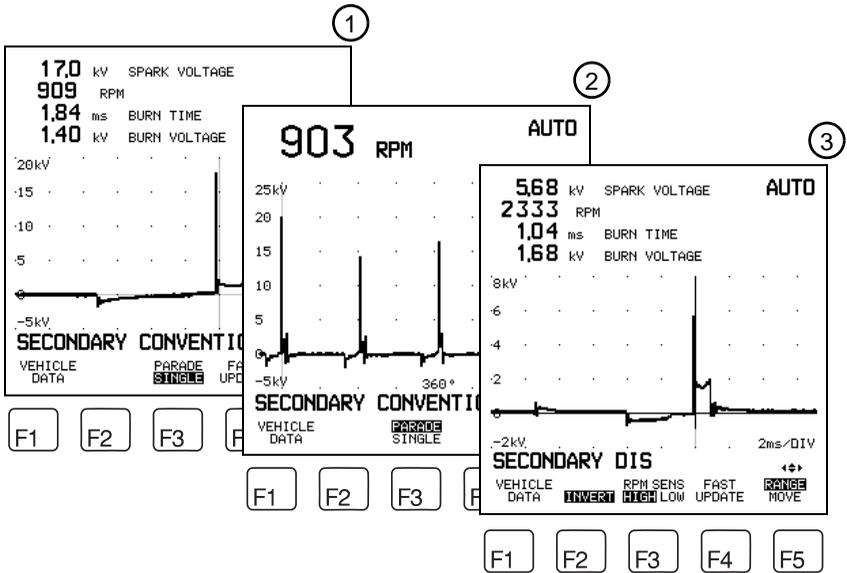
Press this key to invert the displayed ignition waveform.
