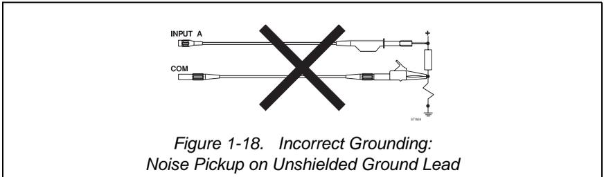
*Figure 1-18. Incorrect Grounding: Noise Pickup on Unshielded Ground Lead*
