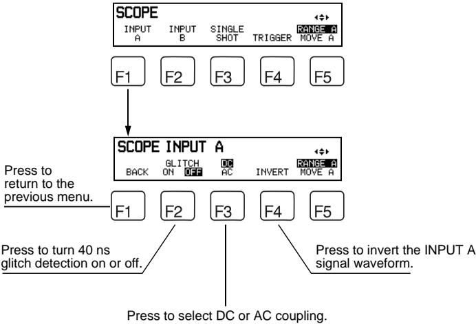
The GLITCH function enables you to capture and display events such as spikes that occur between two samples on INPUT A, which would otherwise not be visible. INPUT B is turned off when the GLITCH function is activated. The events can be glitches or other asynchronous waveforms that are 40 ns or wider. GLITCH detection is not possible in the DUAL INPUT SCOPE function.
