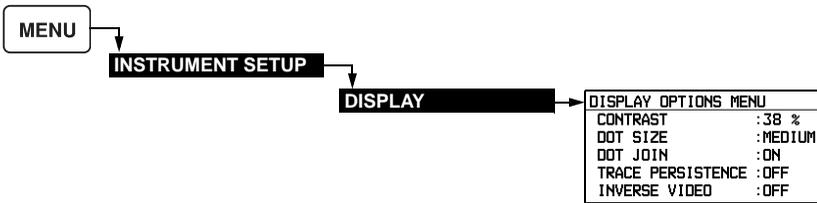
**CONTRAST:** This setting, expressed as a percentage, determines the contrast ratio between display text or graphics and the LCD background.
