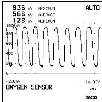
Figure 5-4. Result Display from an Oxygen Sensor Test.
