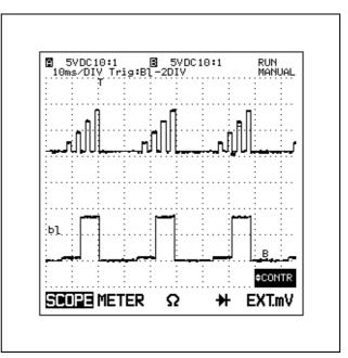
Figure 8-10 Stable Triggering on INPUT B
