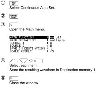
In Figure 7-7, INPUT A represents the current measurement, INPUT B the voltage measurement, and Destination memory 1 the product (equals power).
