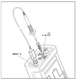
Figure 9-2 INPUT A Probe Calibration Setup
