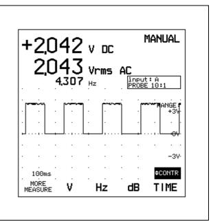
Figure 8-5 Displaying DC Overranging
