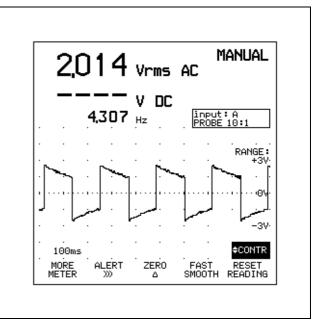
Figure 8-6 Vrms AC Display in Meter Mode
