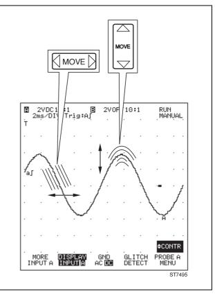
Figure 5-4 Positioning the Waveform
