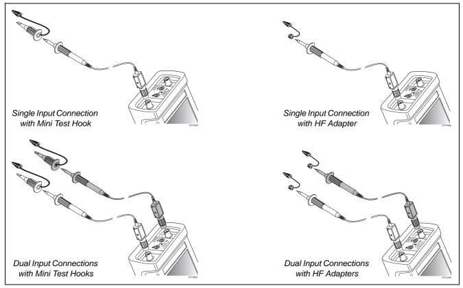
Figure 3 Input Connections for High Frequency Electronic Measurement
