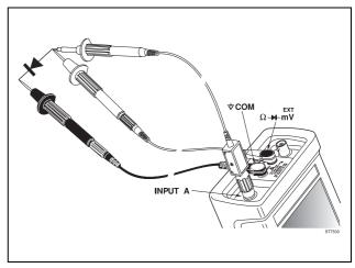
Figure 6-10 Component Test Setup
