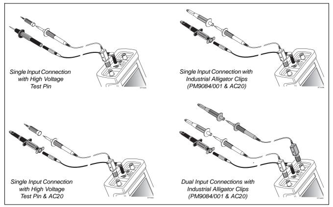
Figure 4 Input Connections for Isolated Heavy Duty Industrial Measurements
