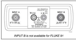
Figure 1-3 Measurement Connections
