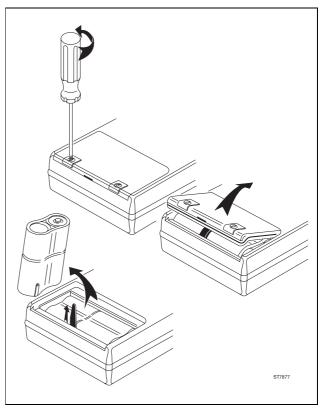
Figure 9-1 Battery Replacement
