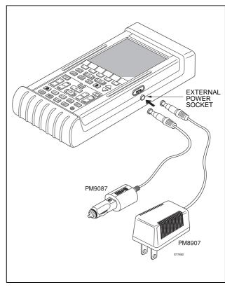
Figure 1-2 Power Connections
