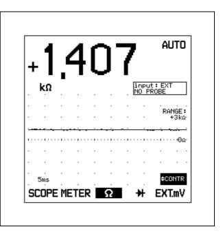
The measurement result is displayed as a 3 2/3-digit display. The ranges are  $30\Omega$  (manual only),  $300\Omega$ , 3 k $\Omega$ ,  $30 k\Omega$ ,  $300 k\Omega$ , 3 M $\Omega$ , and 30 M $\Omega$ . A beeper alert is generated at <5% of a selected range in Manual Range mode. The beeper alert is turned on with ALERT ))).
