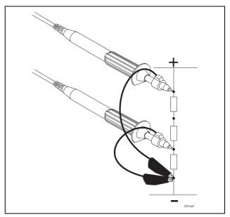
Figure 1 Common (Ground) Connections
