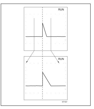
Figure 5-5 Zoom in a Waveform
