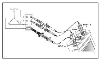
Figure 7-8 Testing a Three-Phase System
