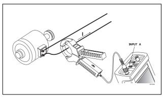
Figure 7-3 Current Measurement Setup
