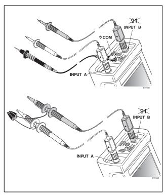
Figure 5-1 Scope Connections
