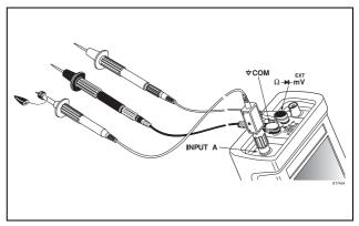
Figure 3-1 Measurement Connections
