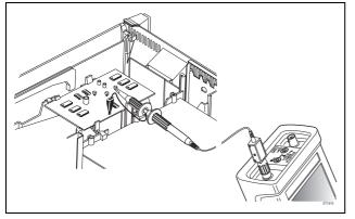
Figure 7-13 Measuring the rise time of a pulse.
