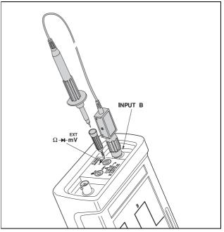
Figure 9-4 INPUT B Probe Calibration Setup
