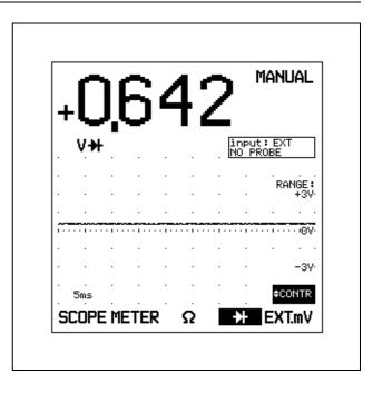
F5 **EXT.mV** EXTernal milliVolt function. Signals supplied to the red and black 4-mm banana jack inputs are measured. The red banana jack is the high input, and the black banana jack (COM) is the low. The ranges are 300 mV, and 3V. Time base ranges are from 1  $\mu$ s to 100 ms/div.
