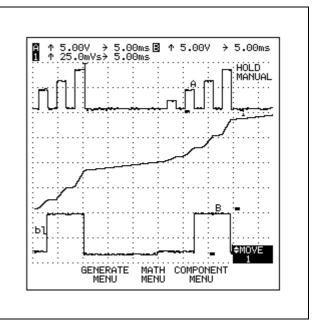
Figure 8-23 Integration of INPUT A
