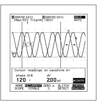
Figure 7-12 Phase Measurement (with Markers)
