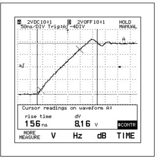
Figure 7-14 Rise Time Measurement (with markers)
