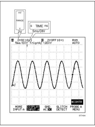
Figure 5-3 Time Base and Amplitude Adjustment
