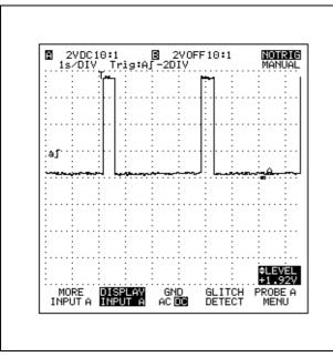
Figure 8-13 Trigger on DC Coupling
