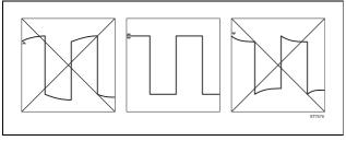
Figure 9-3 Adjusting the Probe
