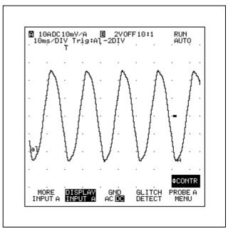
Figure 7-5 Current Measurement in Scope Mode
