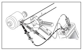
Figure 7-6 Power Measurement Setup
