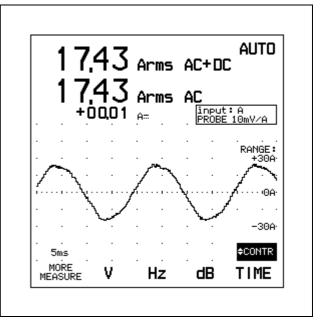
Figure 7-4 Current Measurement in Meter Mode
