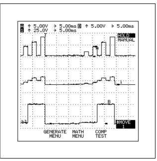
Figure 8-22 Adding INPUT A + B
