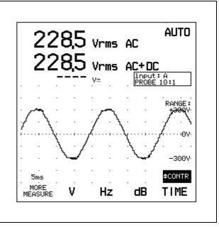
Figure 7-11 AC Volt RMS Measurement
