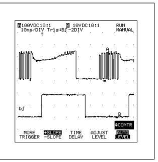
Figure 8-11 PWM Motor Drive Signals
