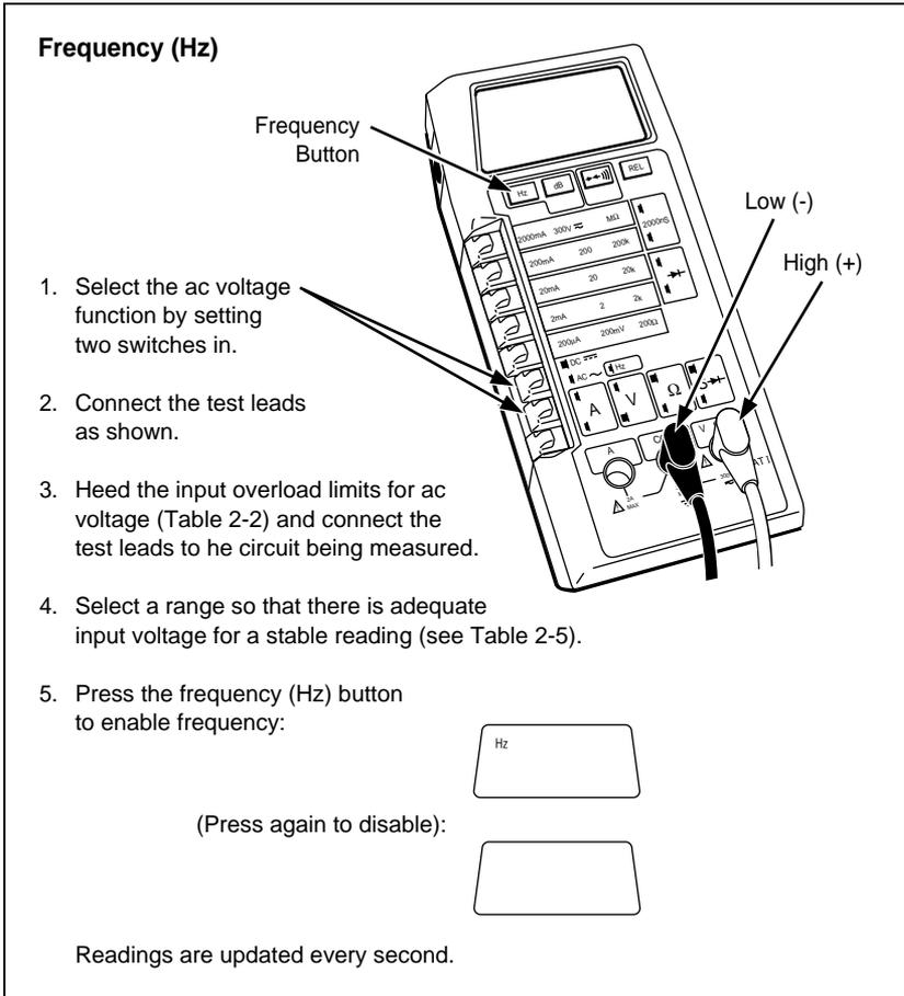
**Figure 2-18. Frequency (Hz) Operation**
