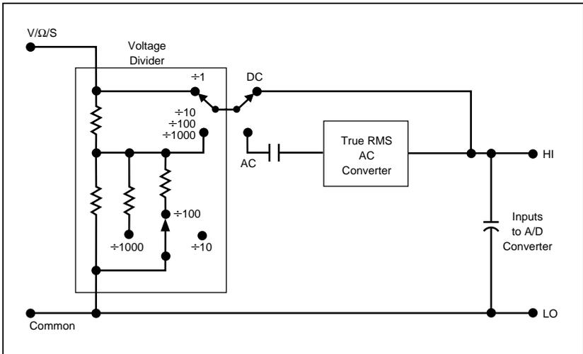
Figure 4-4. Voltage Measurement
