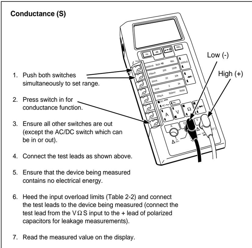
**Figure 2-14. Conductance Operation**
