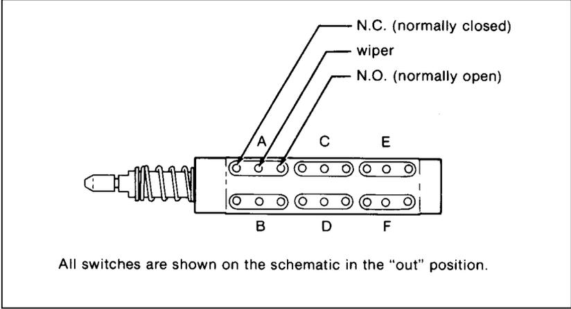
Figure 7-4. Switch Detail
