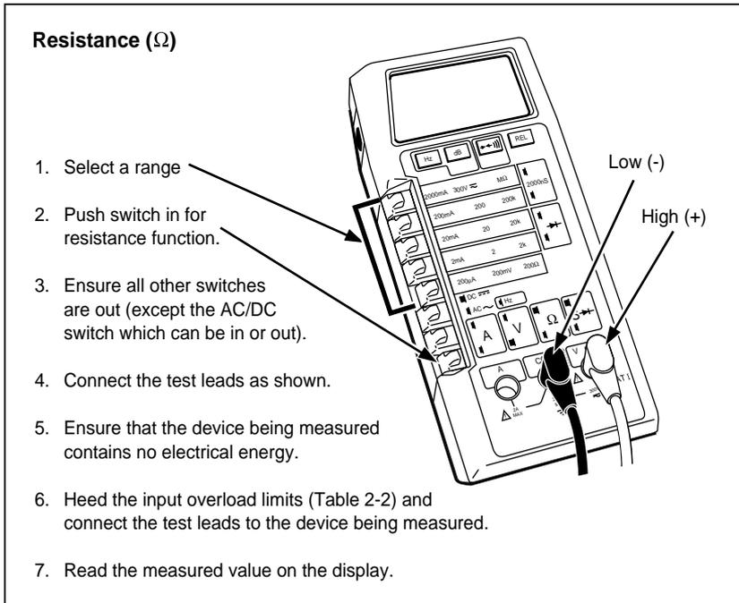
**Figure 2-12. Resistance Operation**
