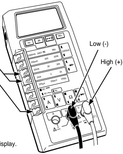
Figure 2-16. Diode Test
